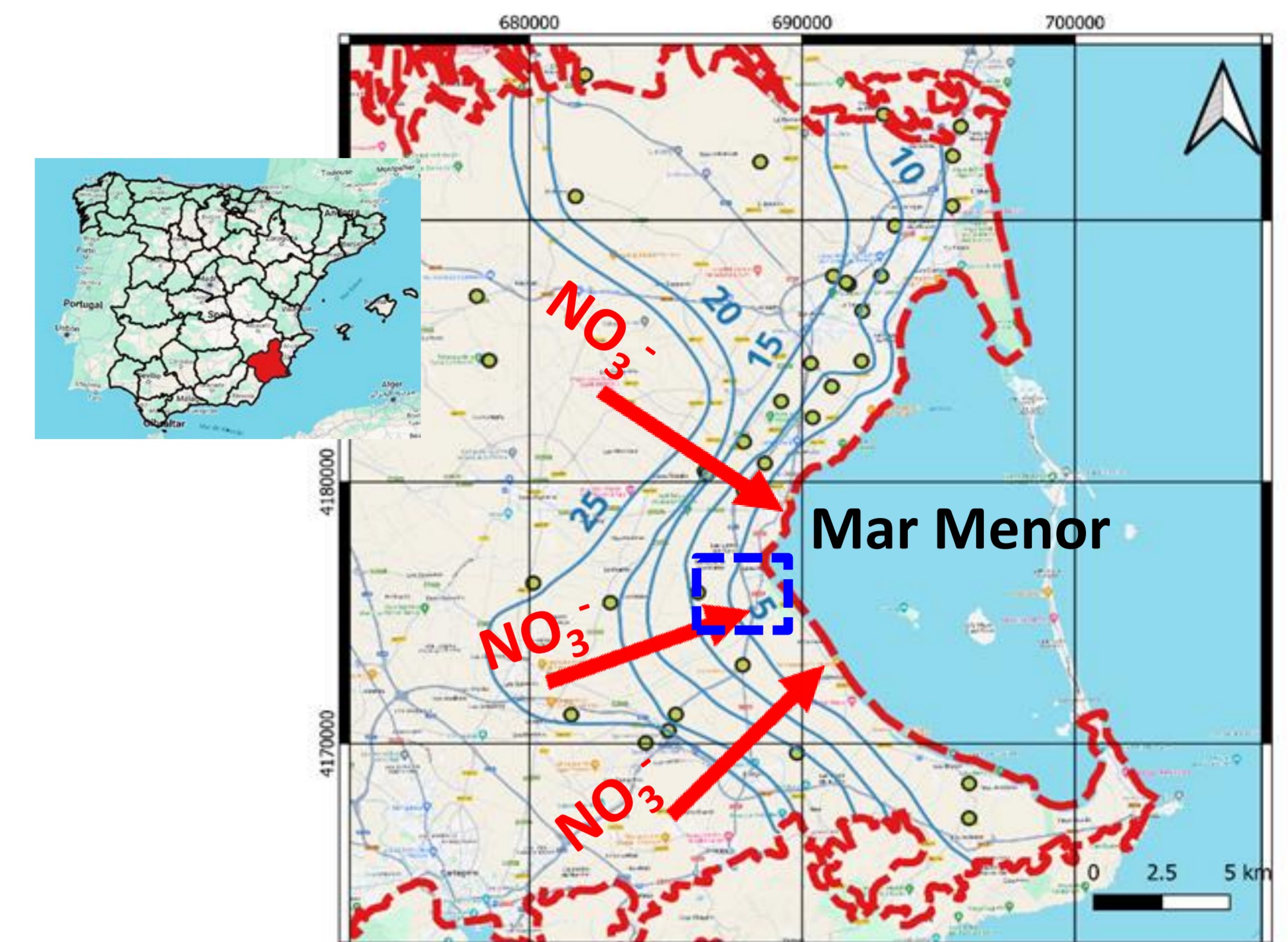
Figure 1. Piezometric map (March 2024) and flux of nitrates discharging by groundwater into the Mar Menor lagoon. Nitrates mainly are related to the agricultural activity in Campo de Cartagena. The blue square indicates the location of the pilot monitoring wells for denitrification of groundwater.
